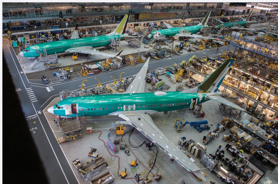
Boeing 737 Max jets undergo final assembly in Renton, Washington.
